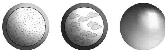
Fig. 1. Schematic drawing of Microcapsules and Microspheres. From left to right: Microcapsule with solution as core, Microcapsule with cell suspension as core, Microsphere with matrix encapsulated active agent.
